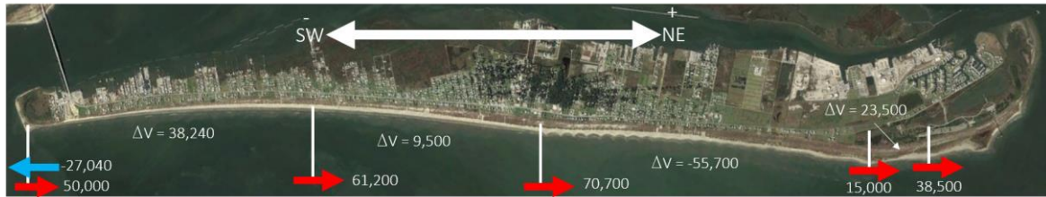
Figure 29. Sediment budget for Grand Isle for existing conditions (units in cy/yr).
