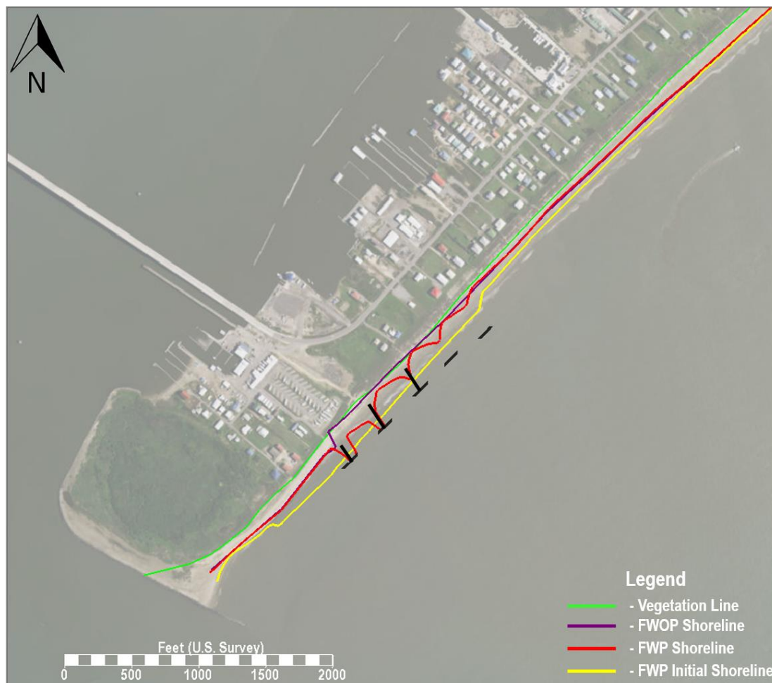
Figure 56. Shoreline response for Alt 4B_v1 at the model timestep when the shoreline hits the vegetation line (9.8 years). Vegetation line (green), FWOP shoreline (purple), FWP shoreline (red), and FWP initial shoreline (yellow).
