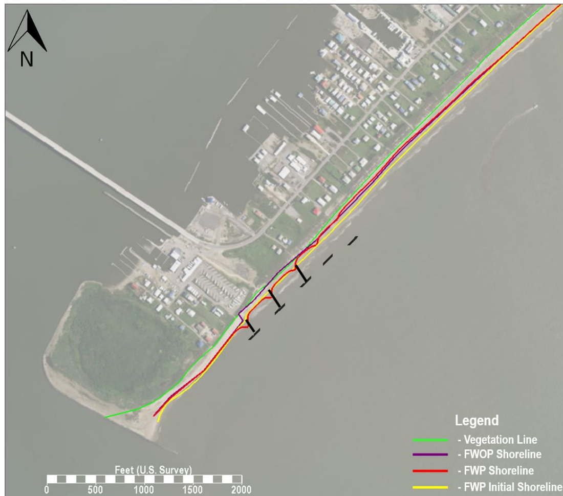
Figure 55. Shoreline response for Alt 4A_v1 at the model timestep when the shoreline hits the vegetation line (7.1 years). Vegetation line (green), FWOP shoreline (purple), FWP shoreline (red), and FWP initial shoreline (yellow).
