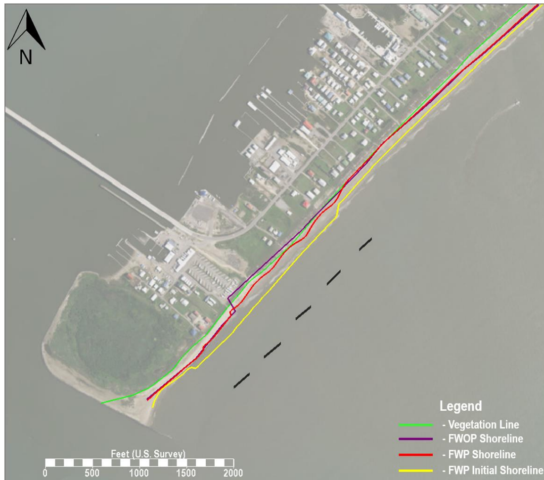
Figure 54. Shoreline response for Alt3B, at the model timestep when the shoreline hits the vegetation line (13.5 years). Vegetation line (green), FWOP shoreline (purple), FWP shoreline (red), and FWP initial shoreline (yellow).
