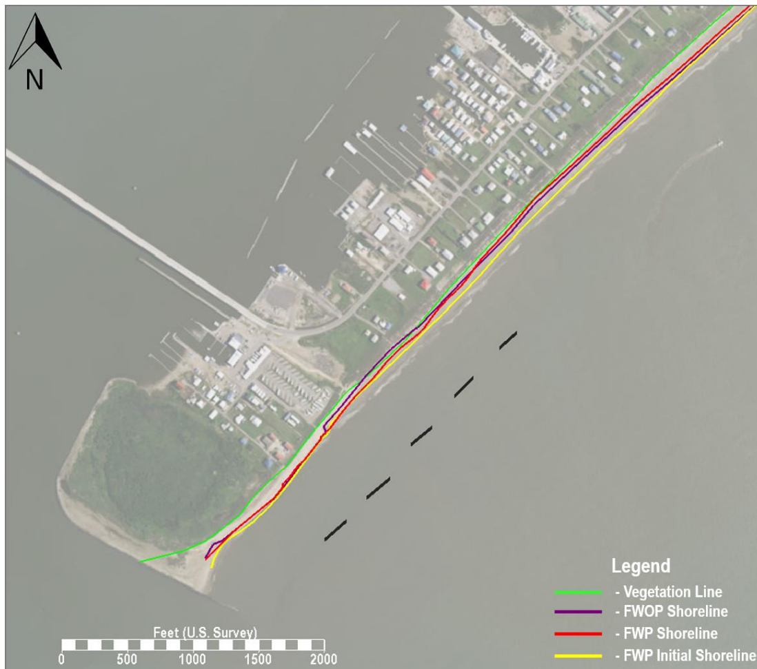
Figure 53. Shoreline response for Alt 3A at the model timestep when the shoreline hits the vegetation line (9.8 years). Vegetation line (green), FWOP shoreline (purple), FWP shoreline (red), and FWP initial shoreline (yellow).
