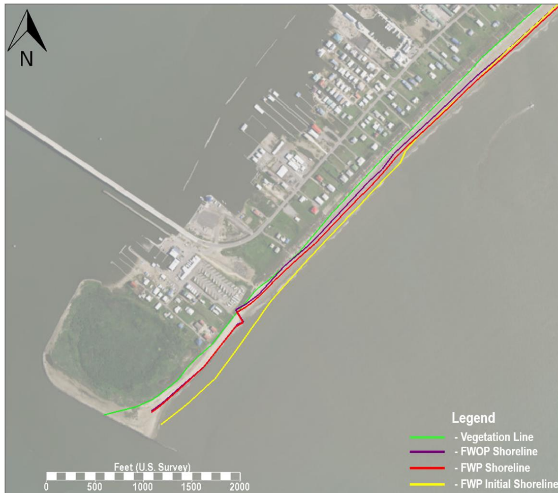
Figure 51. Shoreline response for Alt 2A at the model timestep when the shoreline hits the vegetation line (7.1 years). Vegetation line (green), FWOP shoreline (purple), FWP shoreline (red), and FWP initial shoreline (yellow).
