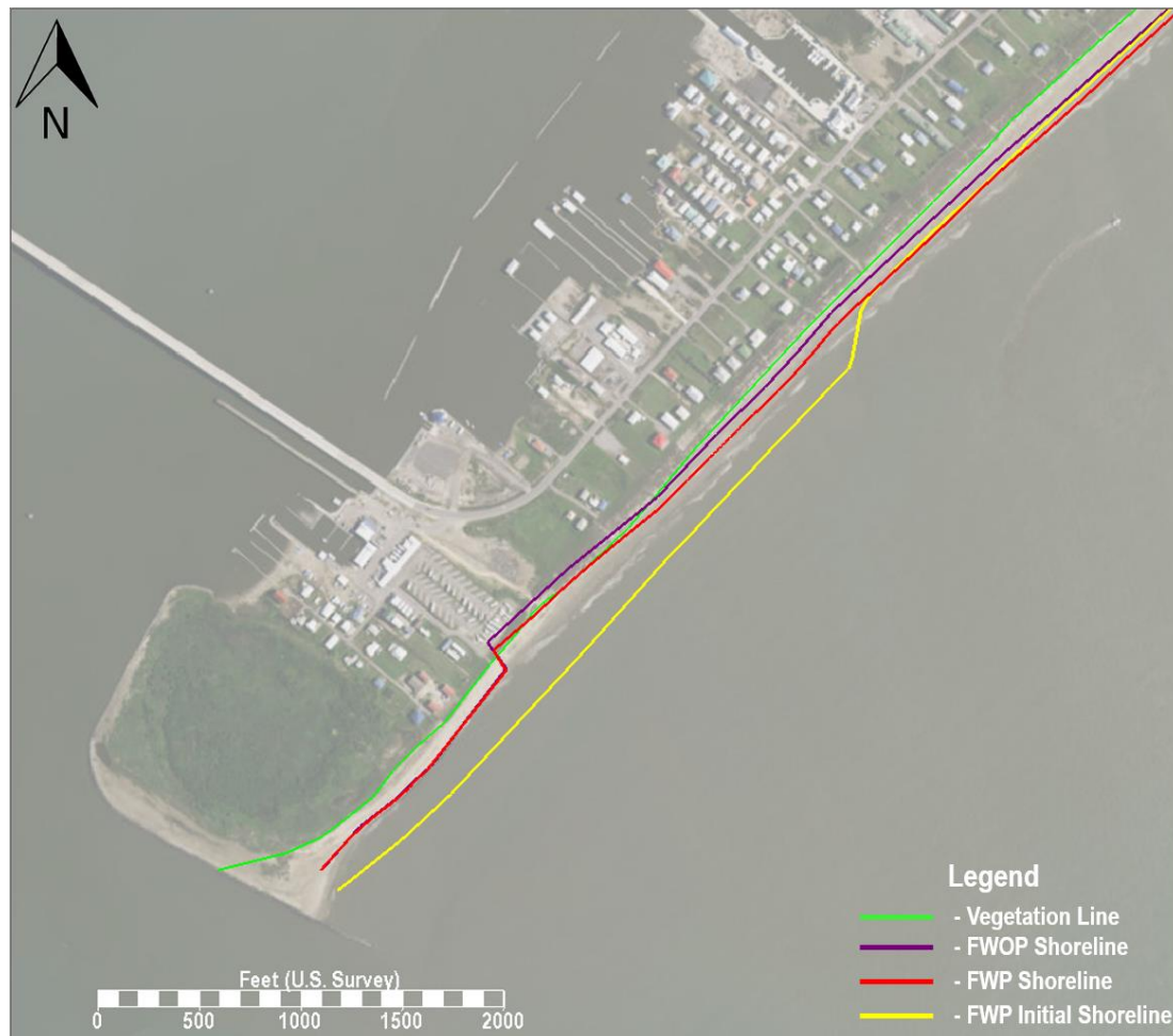
Figure 52. Shoreline response for Alt 2B at the model timestep when the shoreline hits the vegetation line (10.3 years). Vegetation line (green), FWOP shoreline (purple), FWP shoreline (red), and FWP initial shoreline (yellow).
