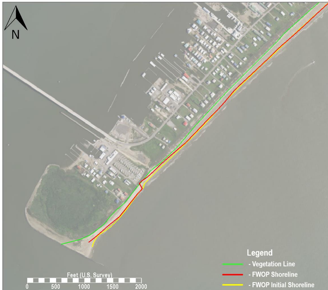
Figure 50. Shoreline response for FWOP/ Alt 1A/ Alt 1B, at the model timestep when the shoreline hits the vegetation line (1.5 years). Vegetation line (green), FWP/ Alt 1A/ Alt 1B shoreline (red), and FWP initial shoreline (yellow).
